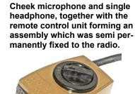
Remote control unit. A led on top of the unit indicated the battery condition.
