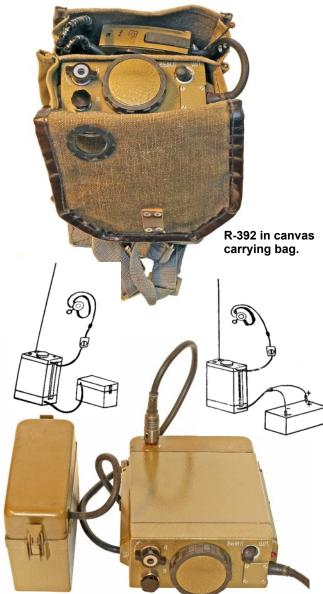
Arrangement for separate carrying the battery close to the body, e.g. in extreme cold, and power from an external 12V battery. (Drawing right)
