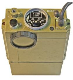
Top view R-392A. Note different (vertical) position of headset assembly cable.
